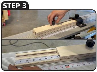
USING KNOB SLIDE BOTTOM STOP OUT TO THE MEASUREMENT CALCULATED IN STEP 2
