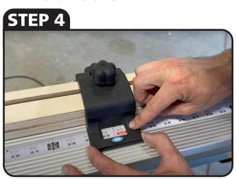
MOVE DOUBLE STOP TO INNER CASING MEASURING FROM DOOR/WINDOW
