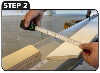
MEASURE CASING WIDTH & MULTIPLY BY 2 EX: 3-1/2" CASING  $\rightarrow 3-1/2$ "  $\times 2 = 7$ "
